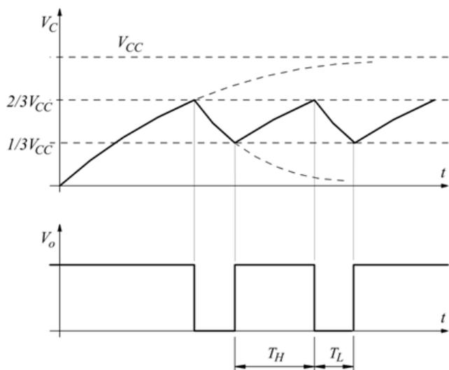
$$T = T_L + T_H = (R_1 + 2R_2)C \ln 2$$
