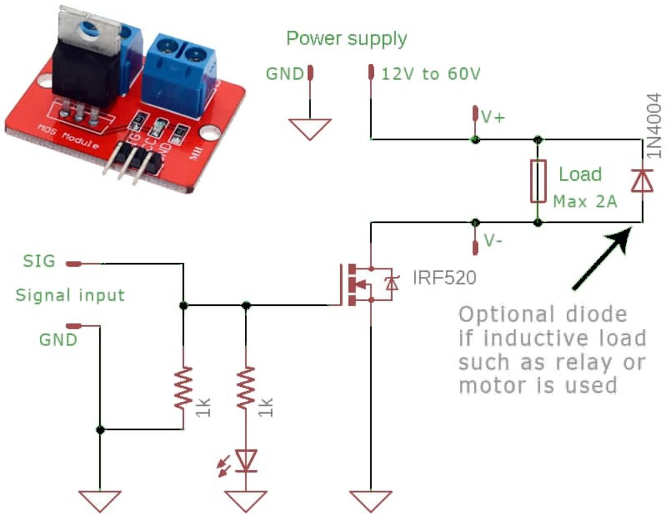
IRF520 MOSFET module can control DC load using Arduino without a relay.
