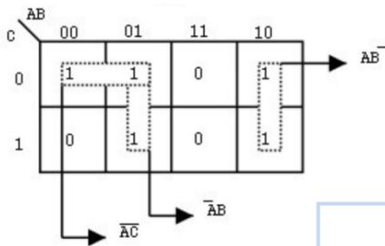
$$Y_a = \bar{A}B + \bar{A}\bar{C} + A\bar{B}$$
