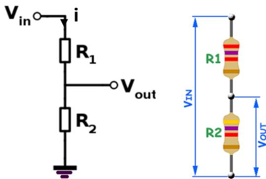
$$V_1 = R_1 \cdot i = R_1 \cdot \frac{V_{in}}{R_1 + R_2} = \frac{R_1}{R_1 + R_2} \cdot V_{in}$$
