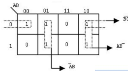
$$Y_b = \bar{A}B + A\bar{B} + \bar{B}\bar{C}$$
