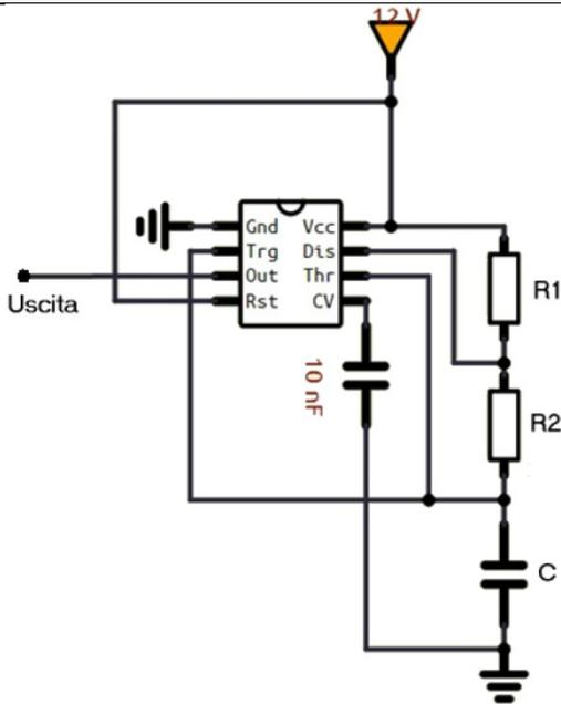
$$T = T_L + T_H = (R_1 + 2R_2)C \ln 2$$
